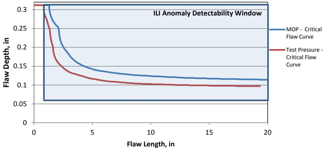
**FIGURE 10.** This chart shows the relative merits of an ILI inspection and an ILI survey by comparing the detectability window and hydrotest and MOP critical flaw curves
