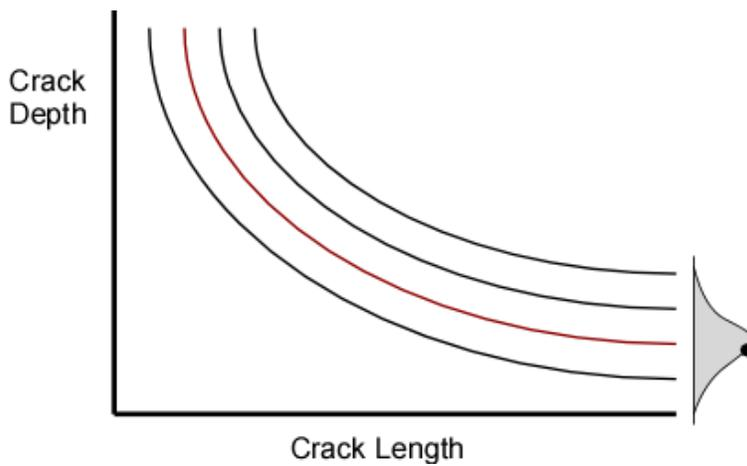
**FIGURE 4.** Family of critical flaw curves for a hydrostatic test, given uncertainty of input parameters to the fracture model. The red curve corresponds to the critical flaw curve selected in a given Monte Carlo trial.
