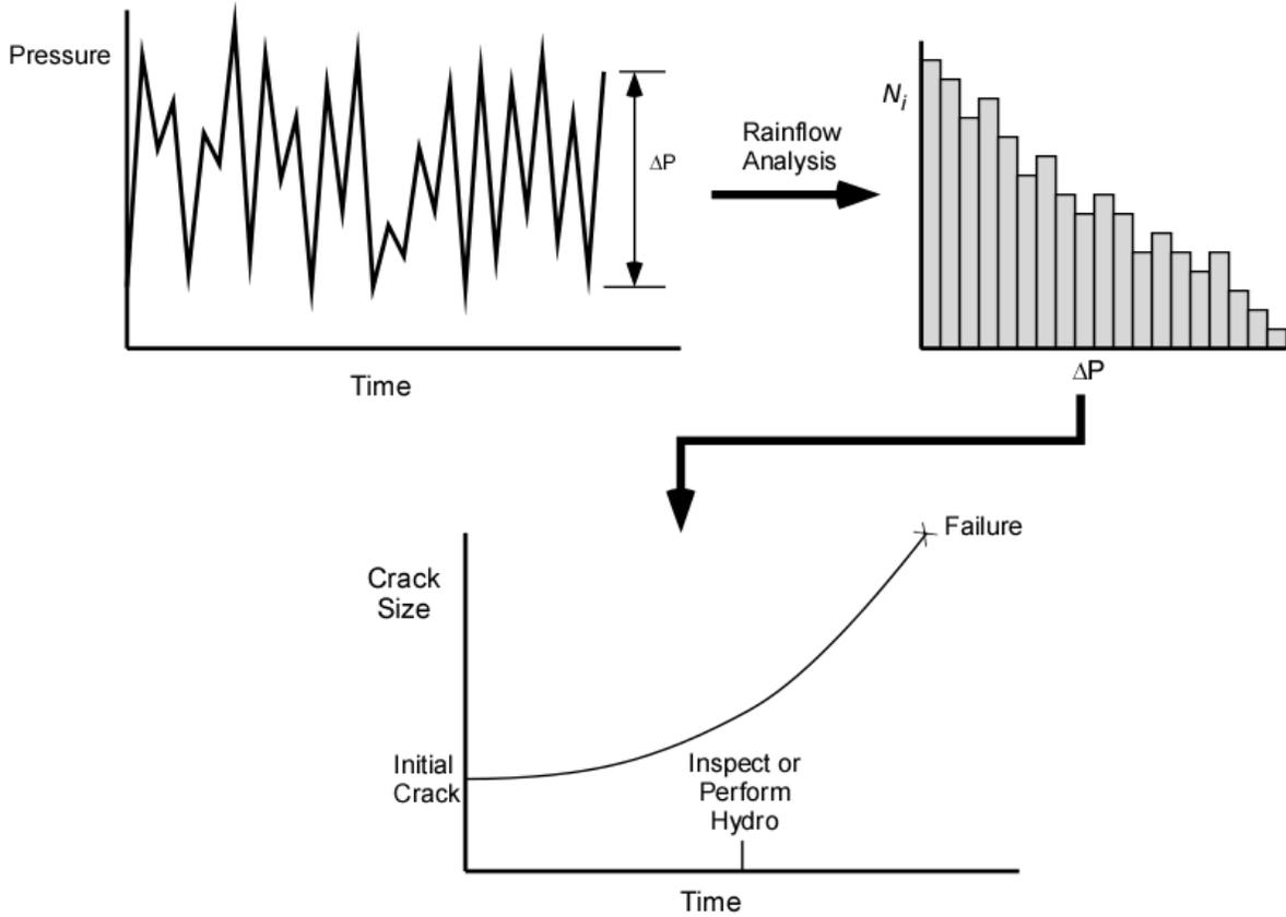
**FIGURE 1.** Pressure cycle fatigue analysis (PCFA). Pressure versus time data are processed through a rainflow cycle counting algorithm to produce a cyclic pressure histogram. This information is then used to predict the growth of a pre-existing crack.
