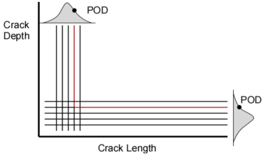
**FIGURE 6.** Determining the maximum undetected flaw length and depth based on probability of detection (POD) specifications for the ILI tool. The red L-shaped curve represents the locus of possible initial flaw dimensions for a given Monte Carlo trial.
