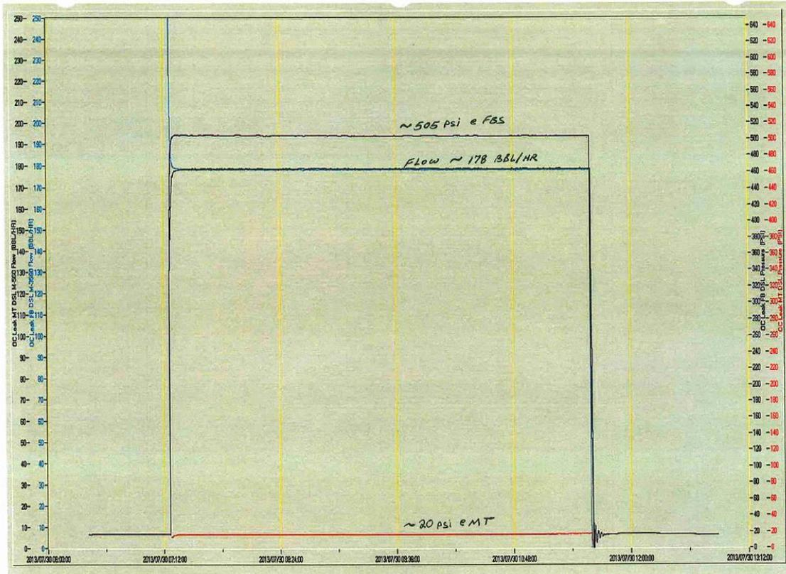
Figure 3. Typical Pipeline Delivery Pressure Trend
