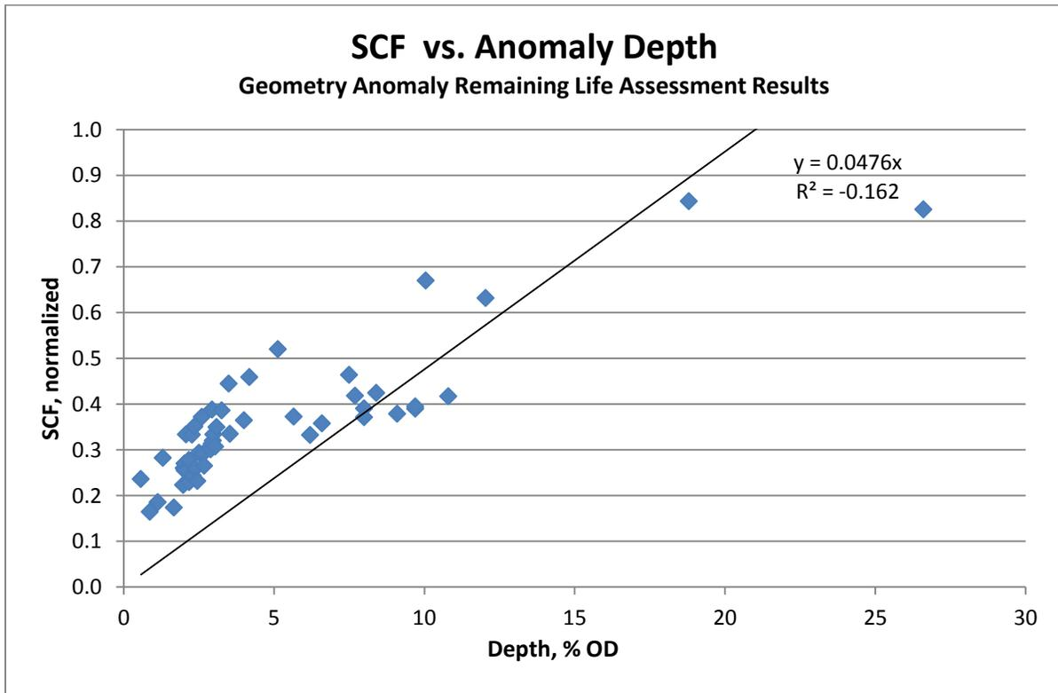
Figure 8. Results of the remaining life assessment: SCF vs. Depth
