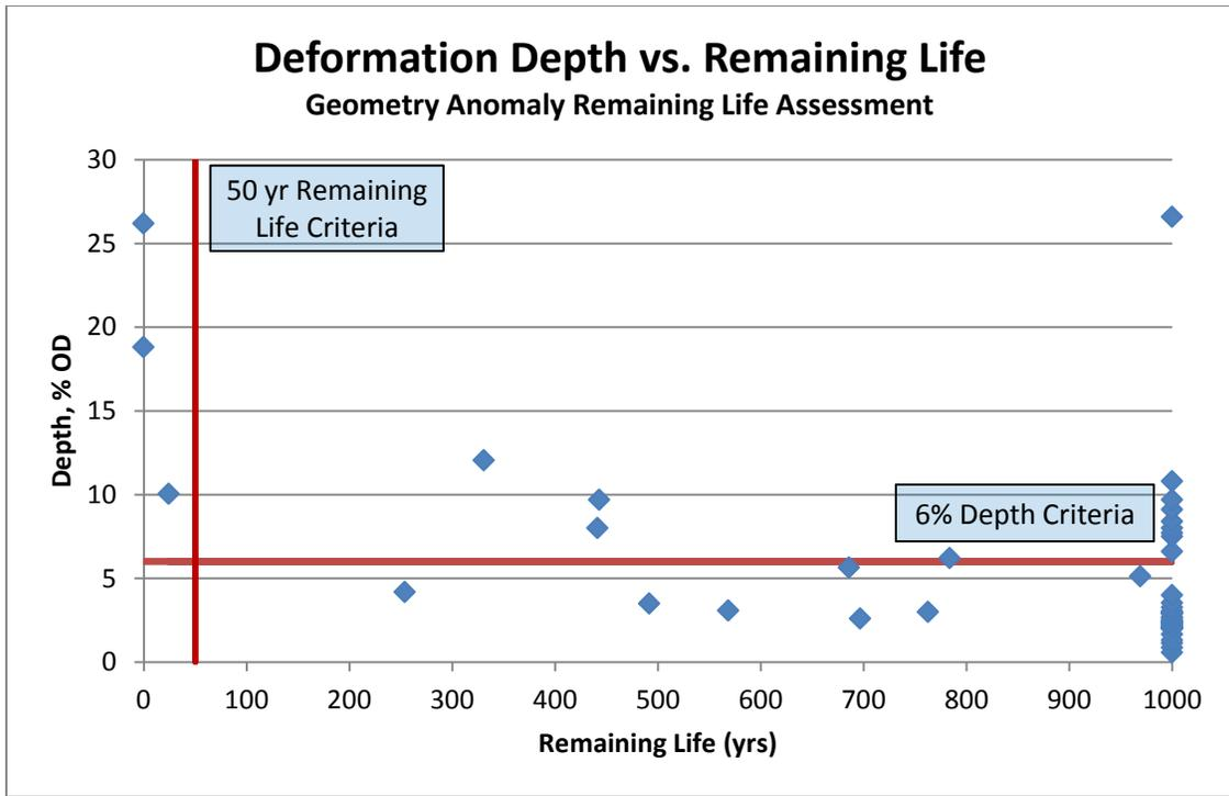
Figure 5. Results of the remaining life assessment: Depth vs. Remaining Life
