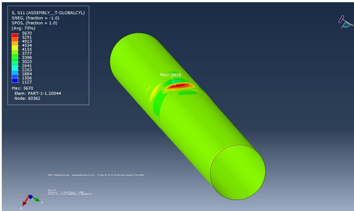
*Figure 4. FEA model of dent showing axial stress due to pressure thrust load*
