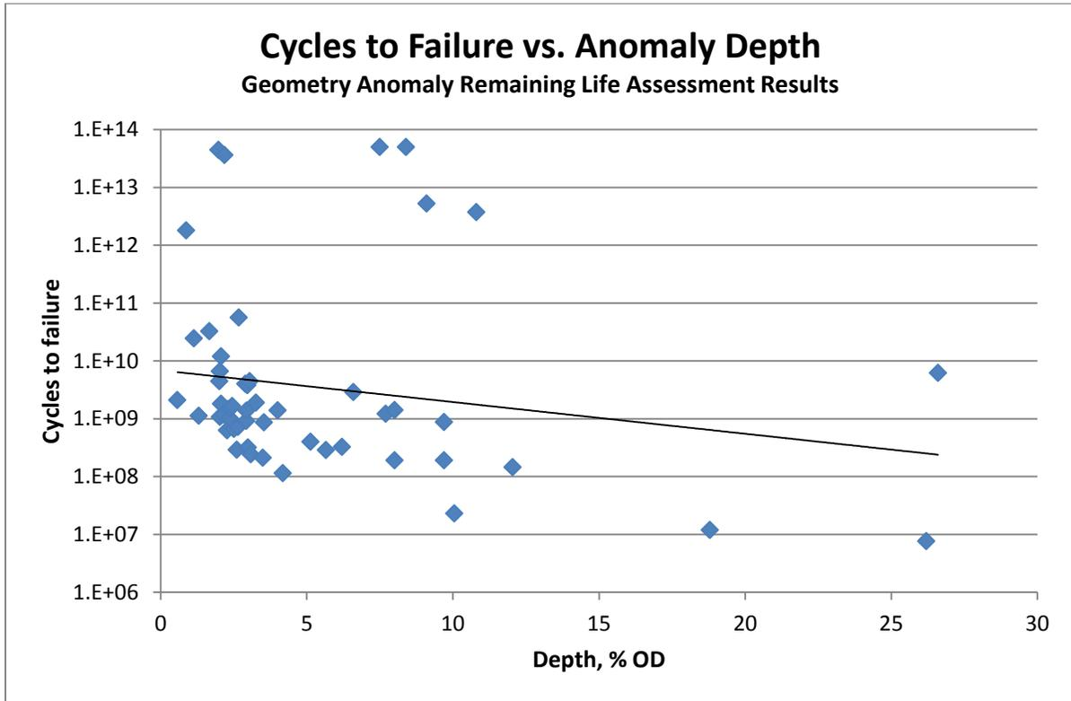
Figure 7. Results of the remaining life assessment: Cycles vs. Depth
