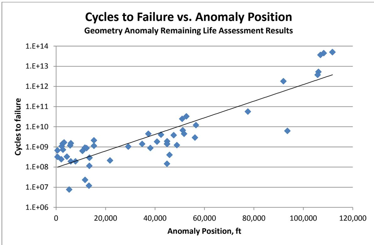
Figure 6. Results of the remaining life assessment: Cycles vs. Position
