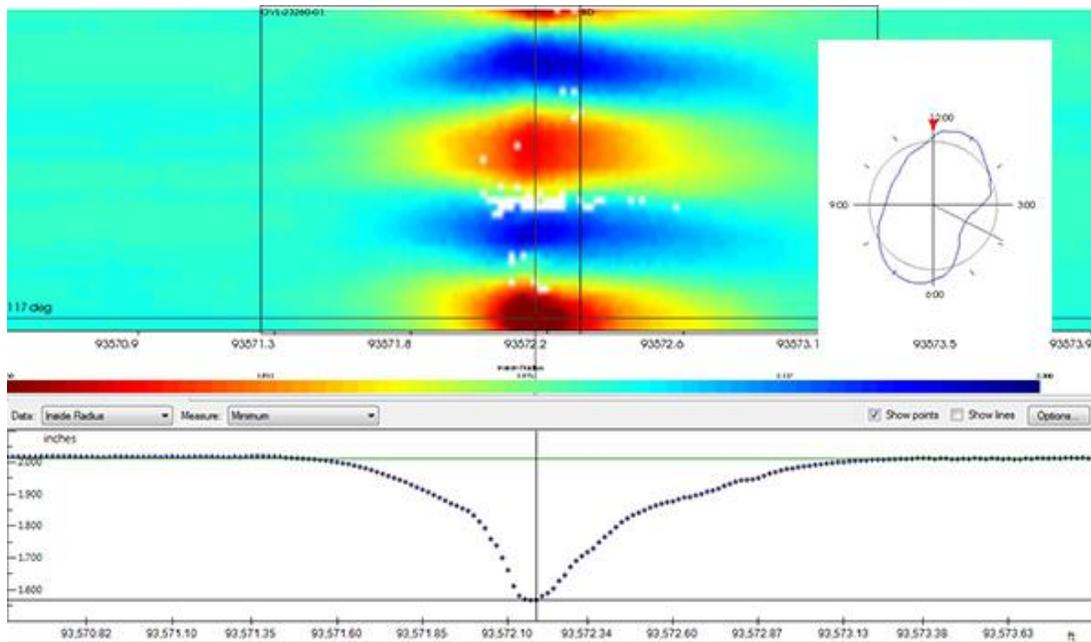
Figure 1. ILI data showing 2D, axial, and cross-section views of 26.6% deep ovality.
