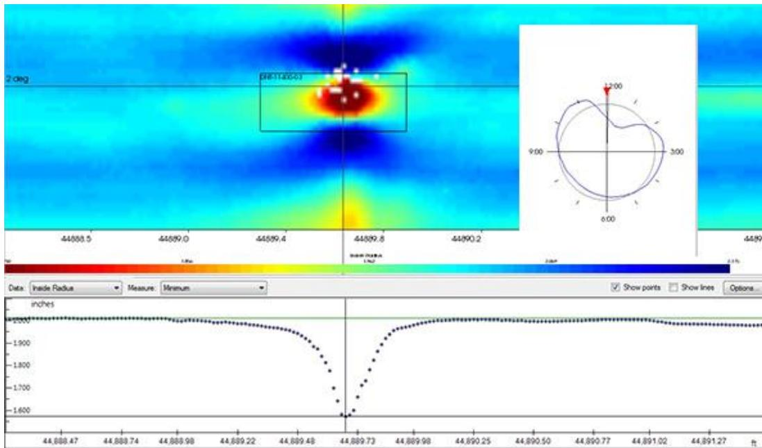
Figure 2. ILI data showing 2D, axial, and cross-section views of 9.8% deep dent.
